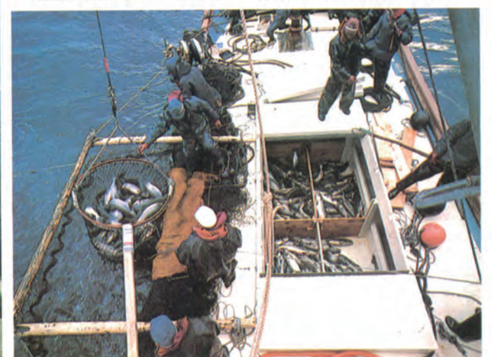
Net hauling. In the main fishing season, several thousand salmon enter the net in a day. Thus, salmon must be transferred into a fish hold with a landing net which is lifted, as shown in the photograph, by a power-driven winch. The fish hold of the Yamaha Fishing Boat DX-199-OA type can accommodate 6,000 salmon (about 2 tons).
