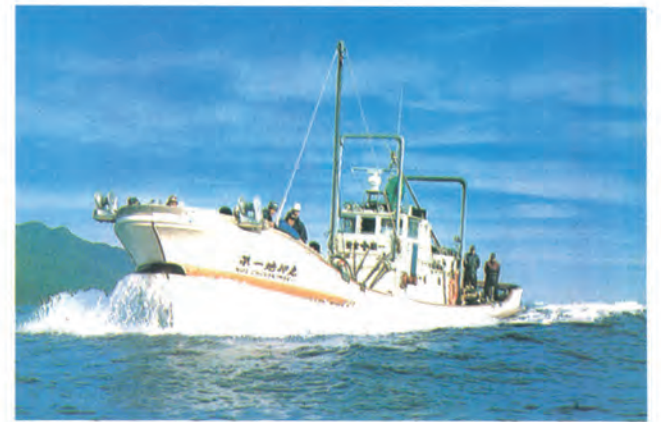
Yamaha Fishing Boat, DX-199-OA Type. This is a fishing boat of 19.9 gross tons used for salmon set net fishing. Four boats are in operation in Hokkaido. Unsurpassed in cruising ability (especially in speed and balance), they are valued highly by each shipowner.
