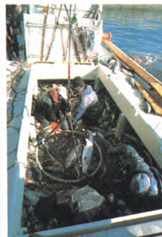
Net hauling. In the main fishing season, several thousand salmon enter the net in a day. Thus, salmon must be transferred into a fish hold with a landing net which is lifted, as shown in the photograph, by a power-driven winch. The fish hold of the Yamaha Fishing Boat DX-199-OA type can accommodate 6,000 salmon (about 2 tons).
