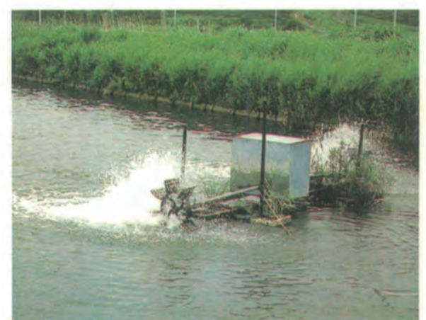
3) Water agitator wheel: Whilst supplying oxygen, this also provides the pond water with a current.
