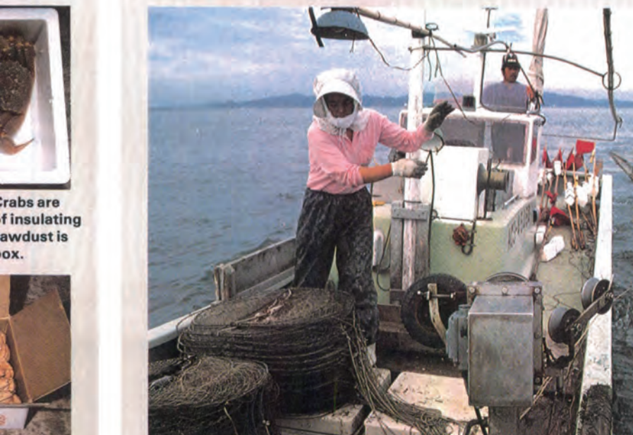
Here, fishing is done by a husband and wife. Because the fishing work is conducted on the front deck, a simple apparatus made of a bamboo pole is devised to operate the throttle lever and the tiller from the anterior side.
