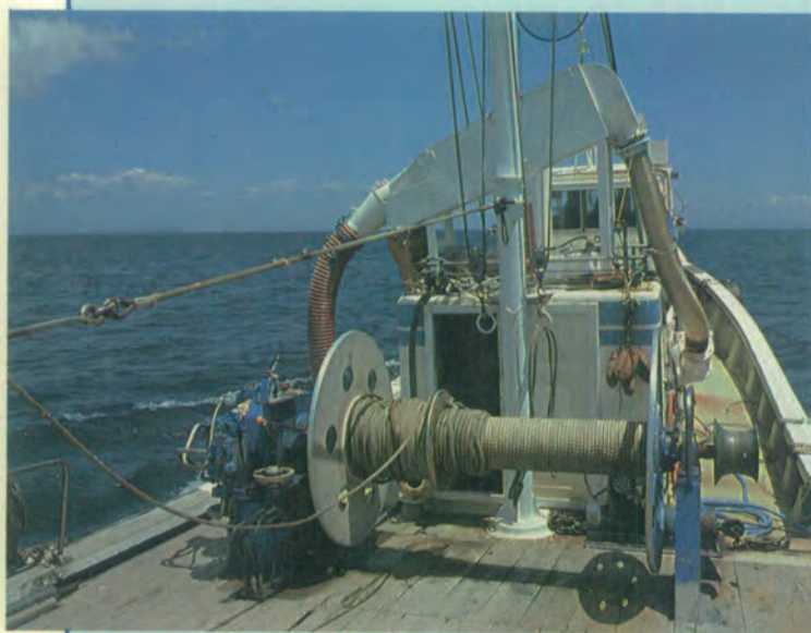
The net hauler seen from the stern. The corrugated pipe seen over the bridge is a fish pump used for especially large catches.
