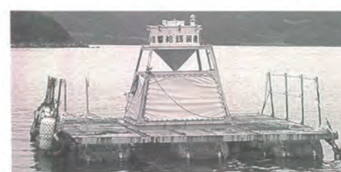
The automatic feeding equipment of this sound-conditioned feeding station runs on batteries and is completely automatic with a feed holding capacity of 7 to 10 days.
