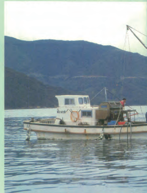
A boat used in the feeding operation. In front of the bridge is a machine for forming moist pellets.
