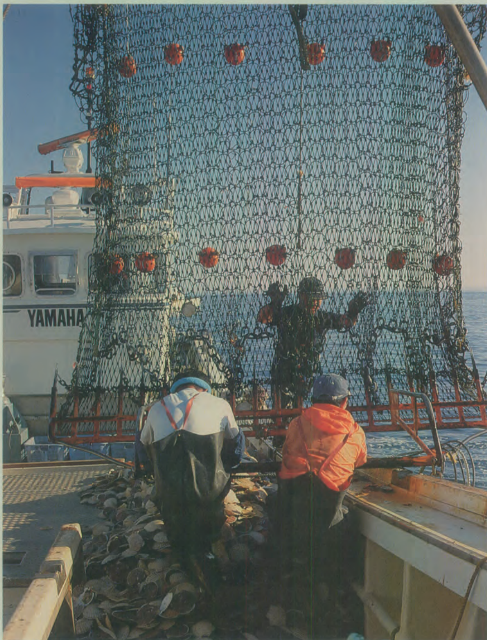
The dredge net measuring 3.3m in width and about 5m in length, the upper net is made of nylon with a mesh of 13.5cm, while the lower net features chains strung to the mouth section of the net and a metal net made of interlocked rings for the portion of the net that drags along the sea bottom.
