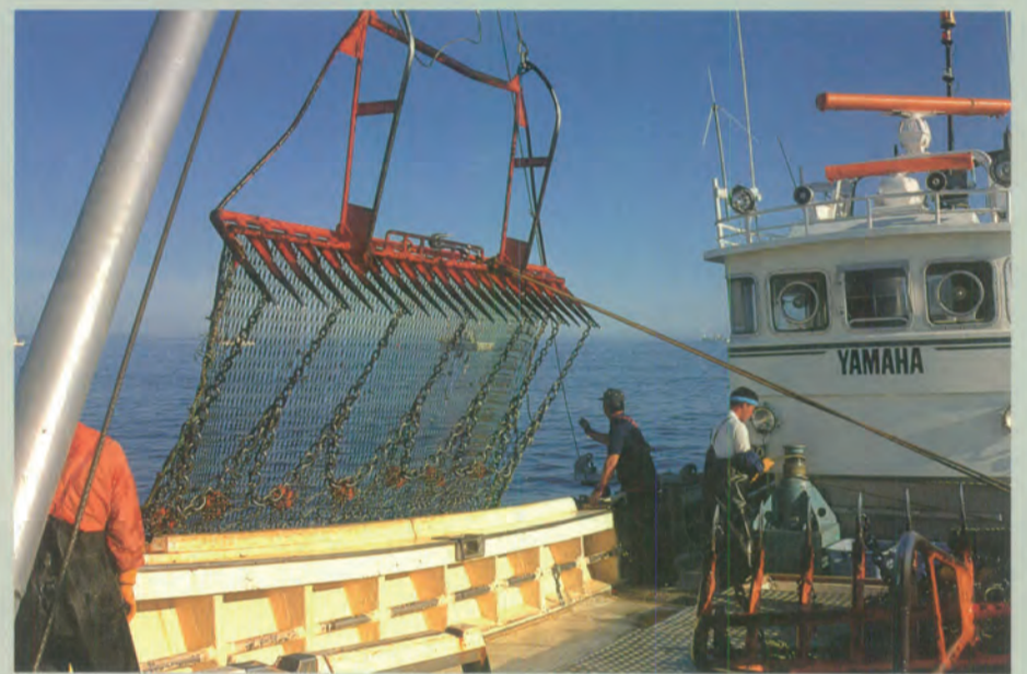
The total weight of the fishing gear is about 350kg. With a 650hp engine the boat pulls two nets, one from each side of the boat.
