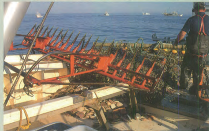
The total weight of the fishing gear is about 350kg. With a 650hp engine the boat pulls two nets, one from each side of the boat.
