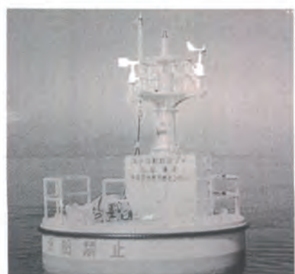
An automatic sea-condition monitoring station (buoy)
